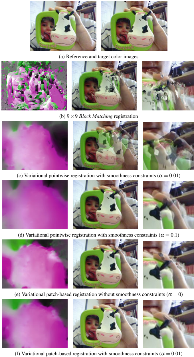
Fig. 3 Illustration of the variational image registration method on the patch space (16), and comparisons with Block Matching and pointwise variational registration (13) methods
