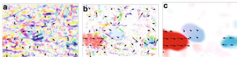
Fig. 3 Result for the Hamburg taxi sequence. (a) Optical flow estimated from the Reichardt detectors k_1 . (b) Optical flow m_1 . (c) Optical flow m_2 . Note the filling in of the left margin due to the activity evoked by the leftward moving car
